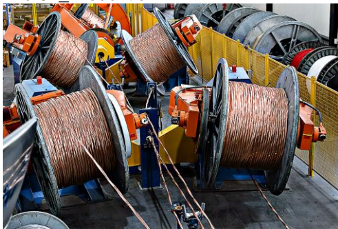
Caption: Universal rope machine in cable production, Brugg site
