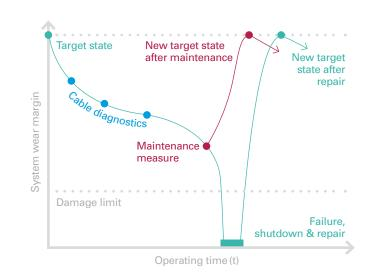
Cable diagnostics help to plan for maintenance measures on time to avoid failures, to prevent shutdowns and to expand the operating time and service life.
