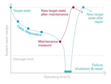
Cable diagnostics help to plan for maintenance measures on time to avoid failures, to prevent shutdowns and to expand the operating time and service life.
