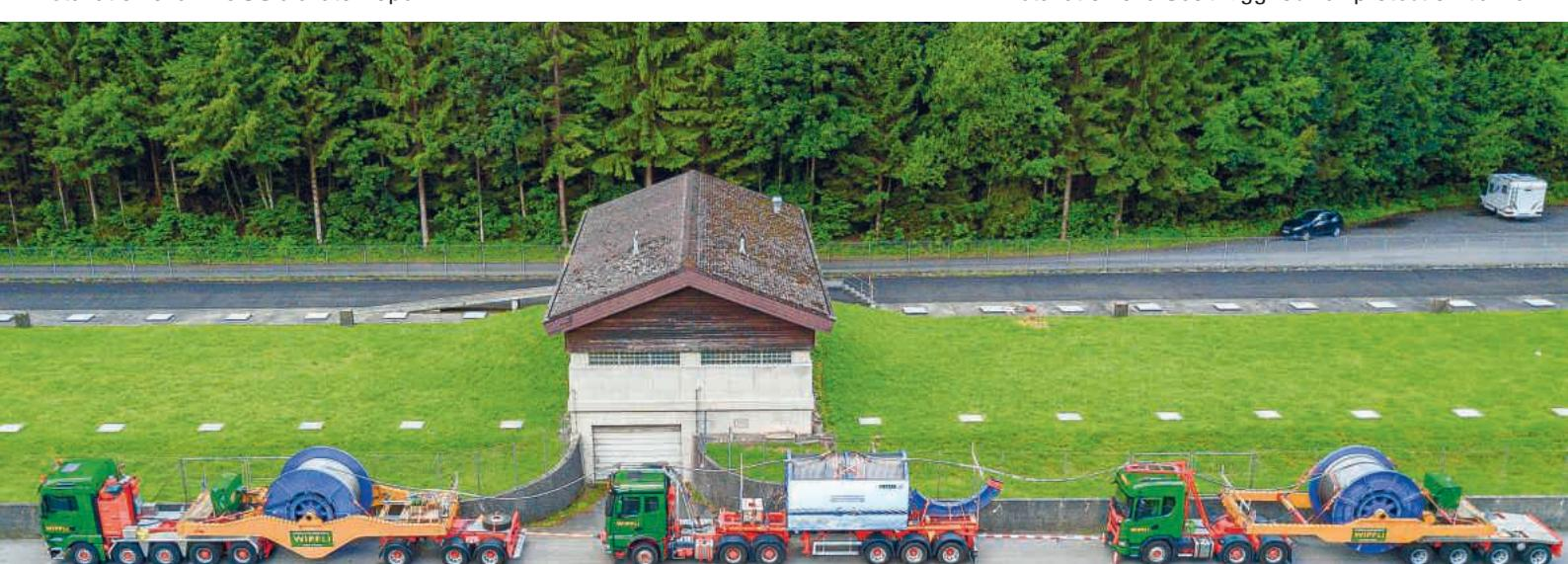
Transportation of a Fatzer track rope on three heavy trucks for the V-Cableway in Grindelwald, Switzerland
