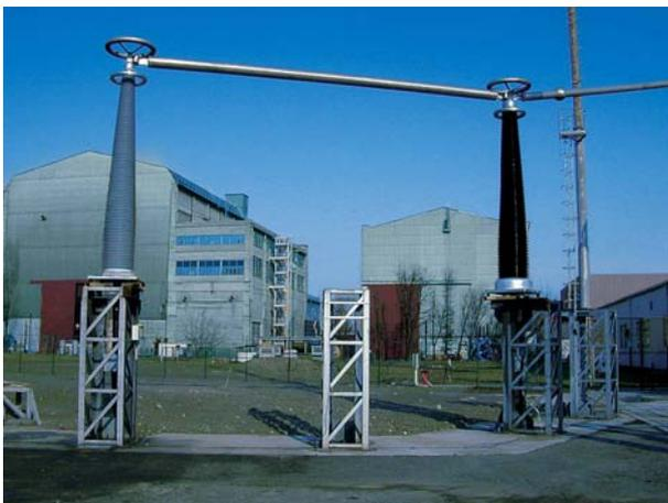
Test Setup of Prequalification Test
