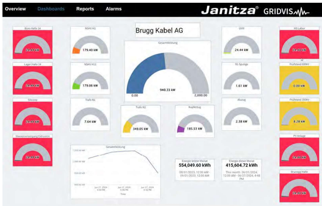
Figure 10 – Screenshot of monitoring system for electricity, water, compressed air
