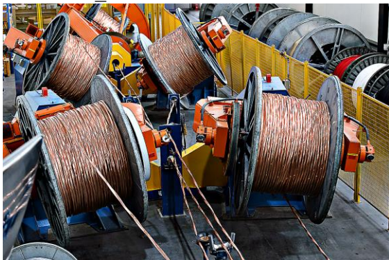
Caption: Universal stranding machine -Cable production site at Brugg
